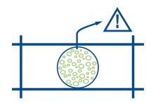
Advanced Phase Measurement accurately measures liquid or gas flow in limited multiphase conditions, providing continuous real-time data at  $\pm 3\%$  accuracy in up to 15% gas-void fraction of gas in liquid and 5% by mass of liquid in gas applications.
