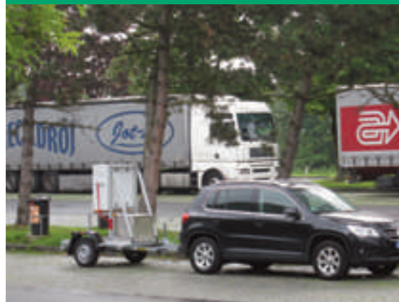
The airpointer can be transported on a pickup truck or a trailer of the right size
