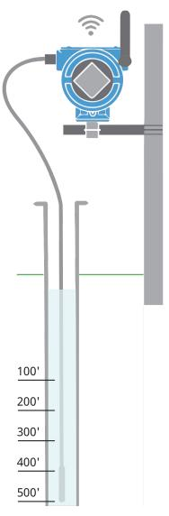
Standard submersible cable lengths up to 500 ft (150 m) can be user modified to specific length on site.
